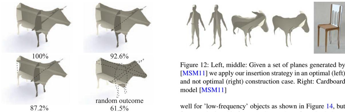
Figure 11: Given a set of planes a number possible outcomes and its insertion area in percentage for a specific insertion order is shown. The random outcome represents the median of 100 random insertion orders. Dashed lines indicate parts that could not be added because of a non-optimal insertion order.
