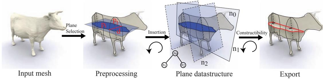
Figure 2: Overview of the construction process. Our pipeline starts with an input mesh. We then perform a preprocessing step which generates a set of polygons that are added iteratively to the cardboard model. By inserting the polygon into our data structure, we split the polygon into individual pieces and efficiently test if those can be physically slid into the cardboard model. If successful the process is finalized by exporting the 2D fabrication plan.
