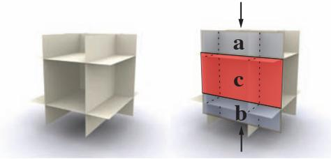
Figure 4: We show an insertion for a symmetric cardboard construction. Note, that the consecutive plane cannot be inserted completely – part  $c$  is physically not insertable. Top and bottom parts  $a$  and  $b$  of the plane can be inserted. Due to symmetry this means that this construction cannot be realized without losing parts of the planes.
