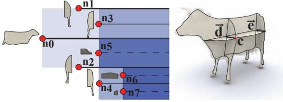
Figure 5: The BSP tree for the cardboard model on the right. The nodes  $n_i$  store its part of the polygon geometry and divide the scene in half-spaces.
