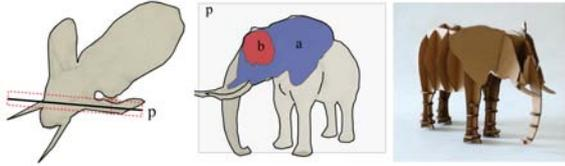
Figure 8: Left: Planar slice  $p$  through the curved ear of the elephant model viewed from above. Middle: Resulting planar slice with point gathering  $a$  and without  $b$ . Right: Fabricated result including the complete elephant ear.
