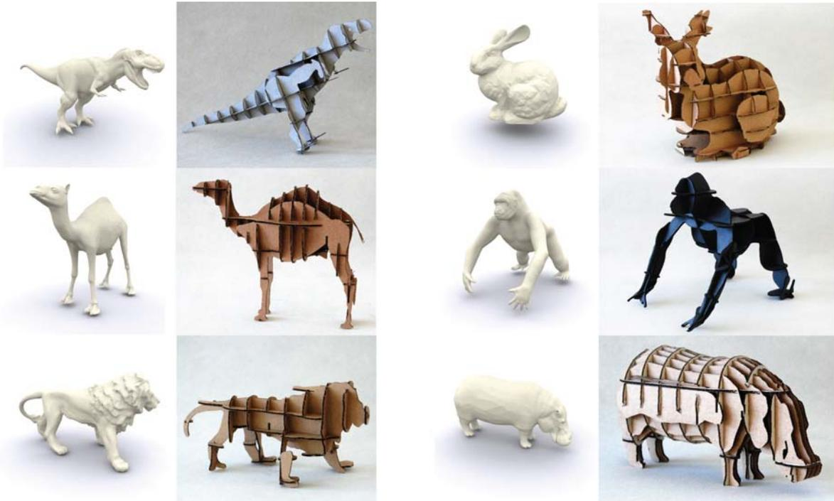
Figure 14: We show the input meshes and the handcrafted cardboard models using axis-aligned grid sampling to find a set of planes. The process for all models is automatic except for the gorilla where we added an additional plane manually.
