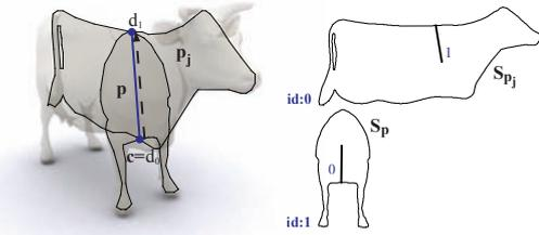
Figure 3: We define  $p_j$  as the *pivot polygon* of  $p$  and  $\vec{d}$  as the *pivot direction* with the *pivot point*  $c$ .  $S_q$  and  $S_p$  define the extracted tiles in the output fabrication plan. We assign each tile an *id* and annotate each slit with the *id* that is connected to the slit.
