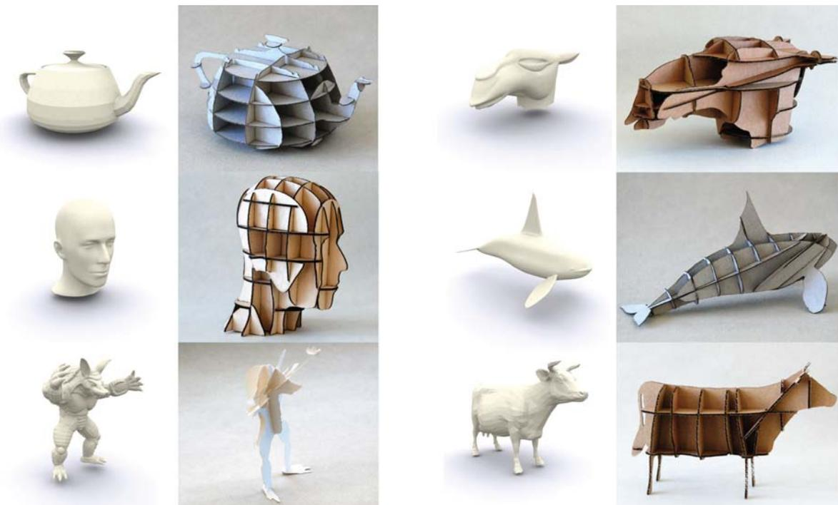
Figure 15: Resulting cardboard sculptures created from a completely automatic two-step process. The first step finds to best *skeleton polygons* using the plane quality evaluation. In the second step we additional sample axis-aligned planes. The Armadillo is created only of skeleton polygons.
