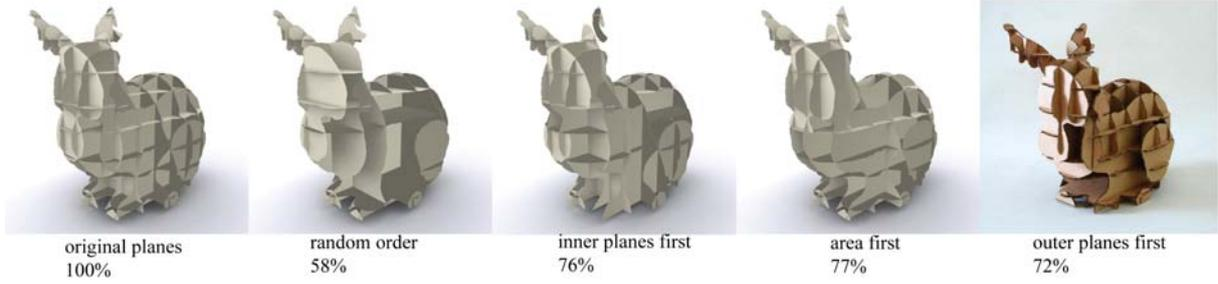
Figure 10: Axis-aligned plane sampling in an 8x8x8 grid. The order of insertion is determined by the decreasing score of the plane. The score is a weighting of area and the polygons distance from the surface. Therewith we control the construction order from inside to outside. If the score is equal for all polygons the insertion is random. It is noticeable that a construction starting with the larger outer planes reconstructs the silhouette much better with nearly the same overall area.
