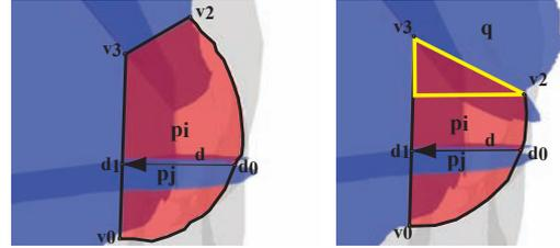
Figure 7: Left: This polygon  $p$  is castable with respect to insertion direction  $\vec{d}$ . Right: The yellow part of polygon  $p$  indicates that it is not castable with respect to the insertion direction  $\vec{d}$ .
