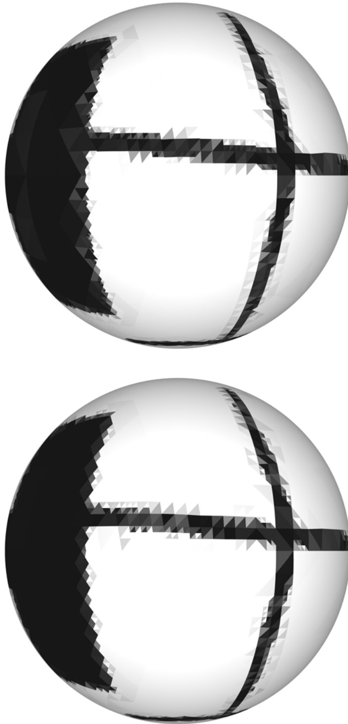
Figure 6.16: Reconstructed visibility map for the SOHO wavelet basis (top) and the Bio-Haar basis (bottom) for an approximation which retained 0.78% of the basis function coefficients of the full signal.
