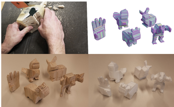
Fig. 11. We test the 'cutability' of optimized cut shapes by cutting various optimized shapes using a bandsaw (left top and bottom) and a polystyrene foam cutter (bottom right). The references for the cut shapes are at the top right.
